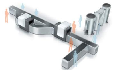
Future Airport Checkpoint X-Ray concept uses same imaging module technology Combination Multi-beam CT & Backscatter with automated detection algorithms
