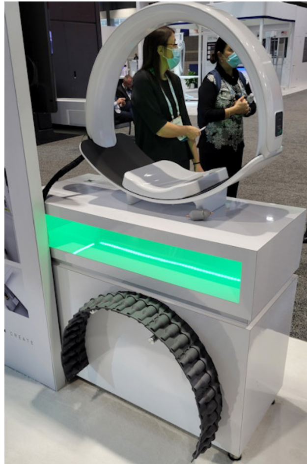
Micro-X is leveraging its carbon nanotube technology into a multisource x-ray system that can be mounted in an ambulance for stroke imaging.
