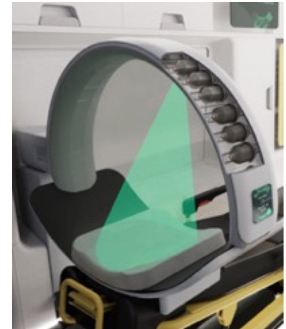
31 miniature x-ray tubes, electronically switched
