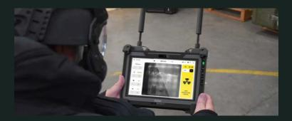
The proprietary software functionality has been designed by operators to be intuitive and easy to navigate. The IR Range Finder provides a visual measuring capability, and user profiles allow images and task narrative to be saved for evidentiary purposes.
